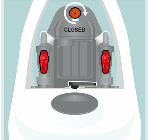
During normal circulation of water through the system during a power flush, both ISOLATING VALVES 1 & 2 should be pointing downward.
