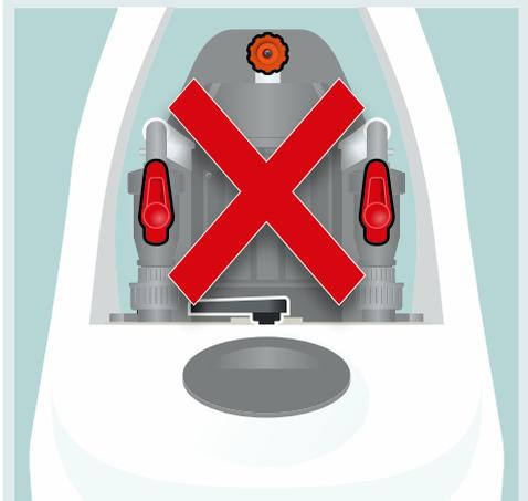
During discharging/dumping, only one ISOLATING VALVE should be rotated into dumping position. NEVER BOTH VALVES.
